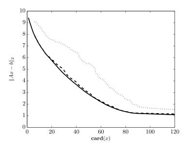
Fig. 11.8. Fit versus cardinality for the lasso (dotted line), lasso with posterior least squares fit (dashed line), and regressor selection (solid line).
