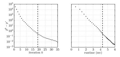
Fig. 11.5. Left. Objective suboptimality of distributed  $\ell_1$  regularized logistic regression versus iteration. Right. Progress versus elapsed time. The stopping criterion is satisfied at iteration 19, indicated by the vertical dashed line.
