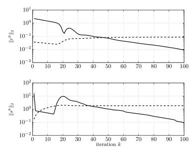
Fig. 11.6. Norms of primal residual (top) and dual residual (bottom) versus iteration, for the distributed group lasso problem. The dashed lines show  $\epsilon^{\rm pri}$  (top) and  $\epsilon^{\rm dual}$  (bottom).
